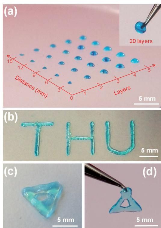
**Figure 2.** 3D printing of polypeptide–DNA hydrogels into 3D structures with a blue dye added for visualization. a) An array of printed droplets with an increasing number of layers (up to 5 layers). Inset: Hydrogel structure with 20 layers. b) The letters “THU” printed with five layers. c, d) A triangle with ten layers, which was printed in five minutes. d) The printed hydrogel structure is strong enough to be picked up with tweezers.
