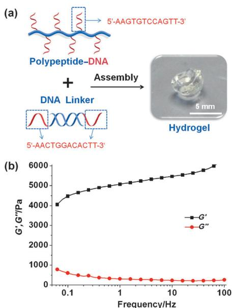
**Figure 1.** a) Preparation of the polypeptide–DNA hydrogel by the two-component mixing of bio-inks **A** and **B**. b) Rheological characterization of a hydrogel (5 wt%). The frequency sweep was carried out between 0.05 and 100 Hz at a fixed strain of 1% at 25 °C.
