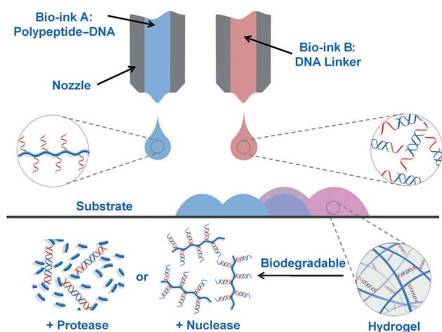
**Scheme 1.** 3D bioprinting of the polypeptide–DNA hydrogel to fabricate arbitrarily designed 3D structures. Bio-ink **A** (blue): polypeptide–DNA, bio-ink **B** (red): DNA linker. The DNA sequences of bio-ink **A** and bio-ink **B** are complementary, and hybridization will cause cross-linking, leading to hydrogel formation (pink). The formed hydrogels are responsive to both proteases and nucleases, resulting in the full on-demand degradation of the hydrogel networks after printing.
